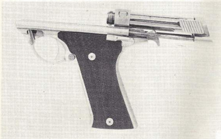
Breech assembly rides rearward on two guide rods, as shown in this disassembled illustration.
