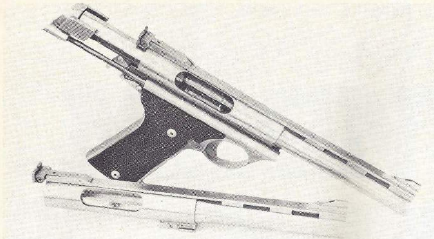
Breech assembly rides rearward on two guide rods, as shown in this disassembled illustration.
