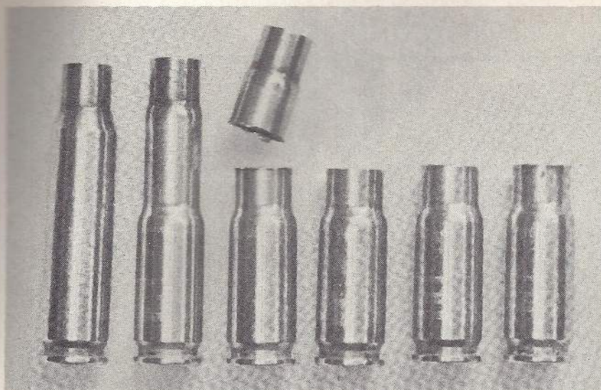
This sequence illustrates the steps necessary to form .357 AMP cases from 7.62mm NATO brass. The case is first run into a form/trim die, the excess is sawed off, then the case is trimmed, neck reamed, resized, and the case mouth is flared. The sectioned cases above, from left, are the trimmed and reamed 7.62mm NATO formed to .44 AMP, and CDM .44; both are suitable for forming to .357 AMP, right.
