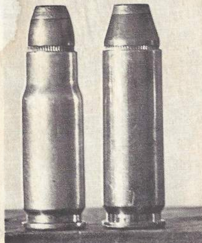
The .357 AMP, left, is made by necking down original .44 AMP.
