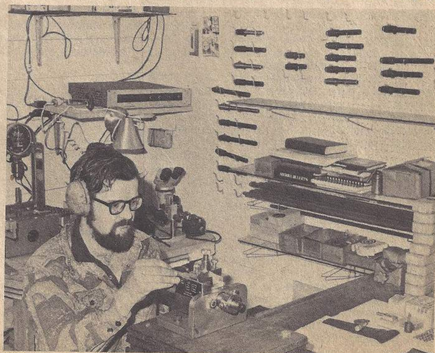
Lomont is one of the niggardly few hand-loader/shooters who have their very own ballistics laboratory set up. Here he prepares to insert copper-crusher cylinder in Phelps-type universal pressure gun. Other pressure barrels are racked on the wall at rear.
