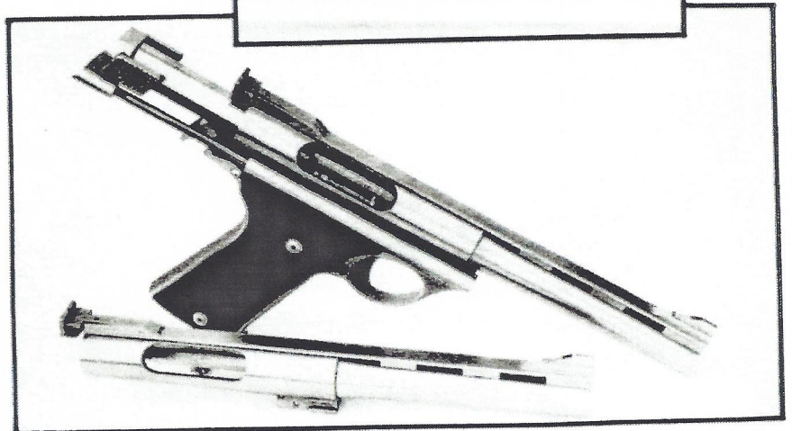
Top: View through right-side ejection port in receiver shows ejector rod and cartridge-enclosing bolt face. Gun barrels of varying lengths and chamberings may be swiftly interchanged without disturbing strike of bullets. New barrels fit old frames.
