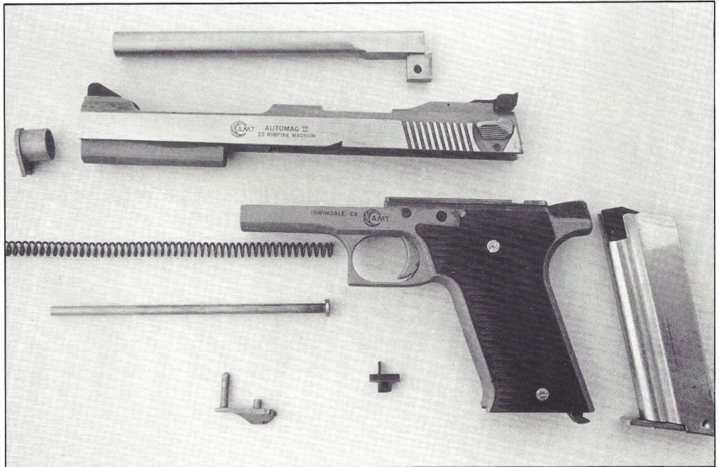
The Automag II field stripped.
