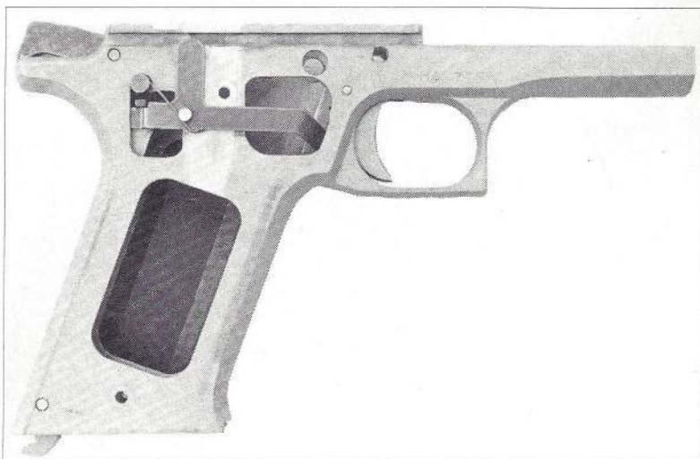
Removing the grips from the frame shows the trigger system and disconnector.
