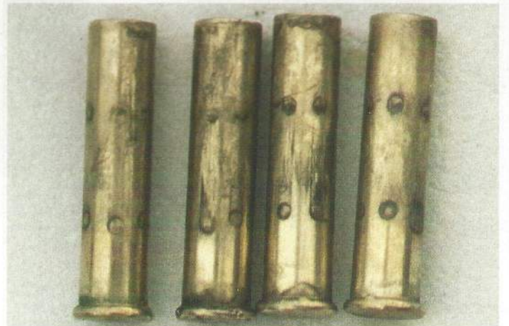
The distinctive signature impressed on the cartridge cases by the Automag's gas assisted system.
