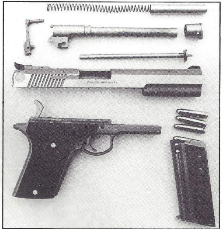
Automag III field stripped. The barrel delay plunger protrudes from the front of the recoil spring guide. Its spring, part CMiB, lurks unseen behind the plunger.
