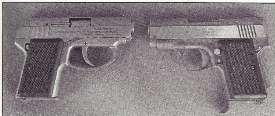
Comparison photo shows redesigned slide and scalloped cut at the rear of chamber for visual inspection. Also prominent is reshaped tang. S/A Backup carries magazine with finger hook extension.
