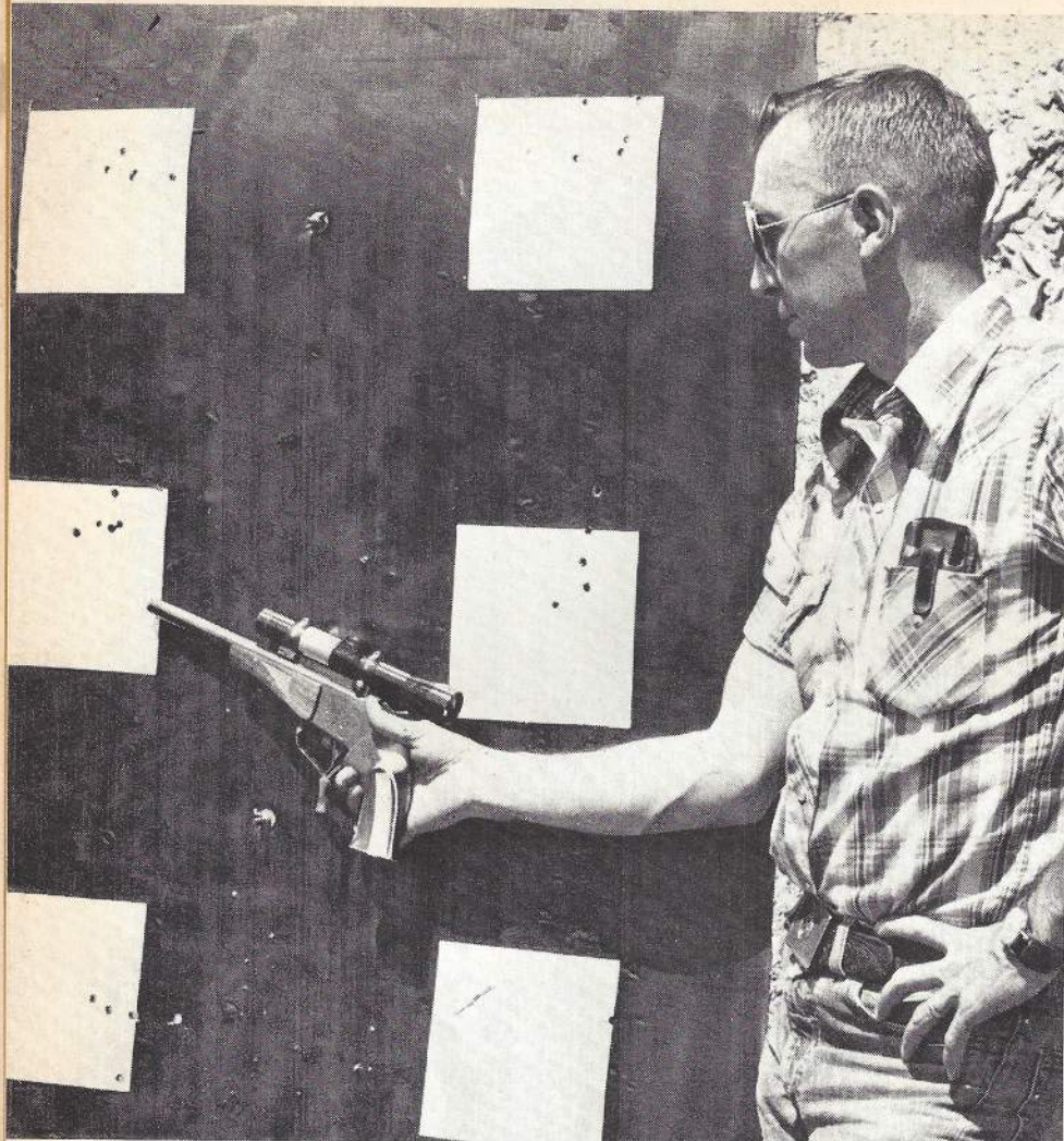
Many long hours and a lot of components go into developing loads for big game hunting. Here, the Author checks 100-yard groups he fired with his .357 Herrett Contender. These were fired in the early stage of load development and each target was fired with a different load.
