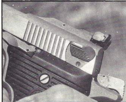
The thumb-operated Automag II safety prevents the hammer from striking the firing pin and blocks the firing pin. It does not prevent the hammer from being dropped when the trigger is pulled. The pistol should never be carried with a round chambered.
