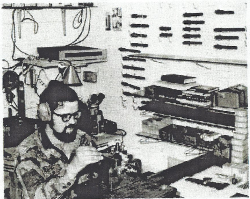
Lomont is one of the niggardly few hand-loader/shooters who have their very own ballistics laboratory set up. Here he prepares to insert copper-crusher cylinder in Phelps-type universal pressure gun. Other pressure barrels are racked on the wall at rear.
