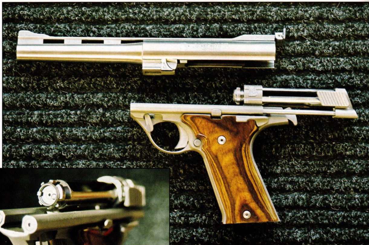
Removing the barrel is effected by retracting the bolt and rotating the barrel latch lever. This permits one to inspect the bolt and the critical locking lugs.
