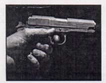
The magazine well is beveled for rapid reloading.
