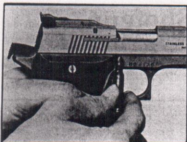
Using a non-marring tool like a bullet point, press out the slide stop to release the barrel from the Automag II's frame.
