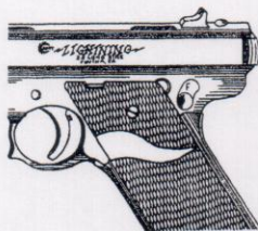
SAFETY IN "OFF" OR "FIRE" POSITION. SAFETY IS ALL THE WAY DOWN.
