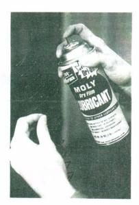
Carefully clean the interior of the magazine and magazine spring, removing all traces of residue and oil. Apply a thin coat of Moly Dry Film Lubricant to the interior of the magazine and the magazine spring. My experience has been in the Auto Mag that this dry film lubricant is superior to any of the oil or grease lubricants. Your magazine is now ready to re-assemble.
