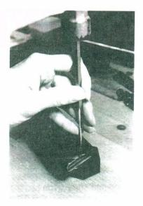
Placing your magazine over a bench block, use a 1/8" punch to remove the follower pin. The pin is serrated and a firm blow is required to remove it. Make note for replacement; the follower pin extends approximately 3/32" from the magazine to engage the arm on the holdpen assembly #34.
