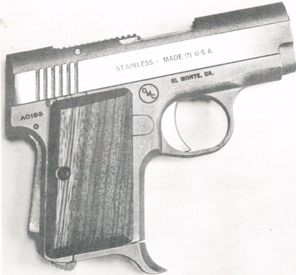
Shown here from the right side, the salient features of the new TDE "Back Up" .380 pocket autoloader are clearly seen. The all stainless exterior is bead blasted to a pleasing matte-grey finish except for the sides of the trigger and the slide flats; the large grip safety pops out to this extent when the hammer is cocked. Grips are smooth-finish walnut nicely inlaid and secured by socket-head screws. The butt-secured magazine carries a curved extension base for additional finger purchase.
