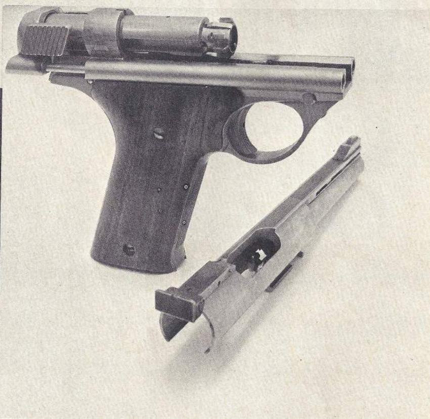
Field-stripping can be accomplished in three seconds. Then, all reciprocating parts are completely open for maintenance. The hole in the center of the grooved trigger is for precise trigger adjustment. Barrel, rib, upper receiver and bolt-locking shoulders are all machined from one piece.
