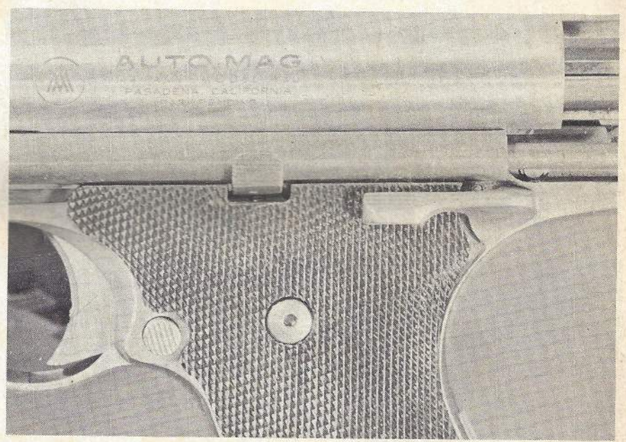
Upper: Details of the extractor, ejector and locking lugs can be seen in this close view of the rotary bolt face. Lower: Controls are on left, convenient for right-handers; hold-open is in center.
