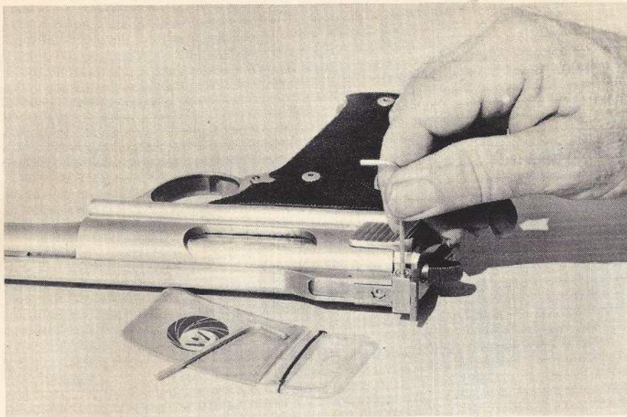
Above: Rear sight adjusts by one of the two hex-wrenches supplied with pistol. Right: Two strips of self-adhesive reflective material, red and yellow, are furnished for use on rear surface of front sight. Below: Foam-lined case affords maximum protection and convenience. It comes with spare magazine, instructions, lube oil, sight insert strips, hex-wrenches and lift-out insert to provide space for plastic ammunition container.
