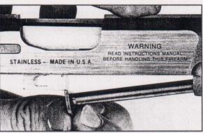
The Automag IV's recoil spring guide is long and is somewhat tricky to extract (recoil spring was removed for clarity).
